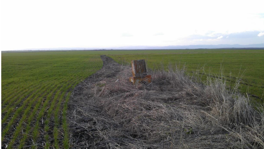
Fig. 3 Unusable triangulation point from the national geodetic network
